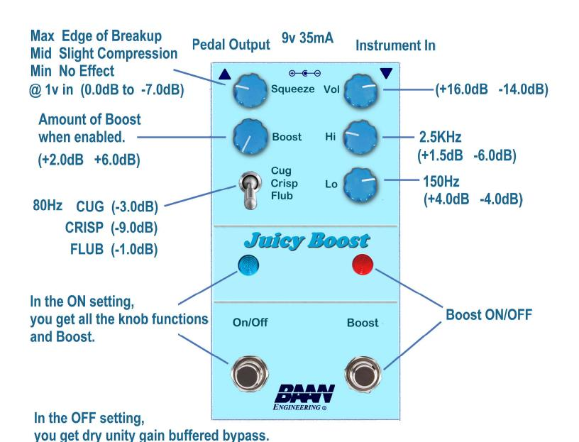
In this setting, none of the knobs or Boost have any effect.
